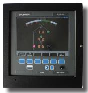
The SKIPPER DL 850 is a dual axis speed log, working on the Doppler principle, providing longitudinal and fore/aft transversal ship speed relative to the sea bed or the water. The DL 850 provides accurate navigation parameters measured as they happen, and presented in a logical, user friendly way.
