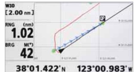
The plotter display traces own ship's track and shows position on a 2-D map\*. This mode presents various data and information with graphic symbols and icons, rather than text. The Auto Waypoint Entry function plots ship's track as "WAYPOINTS". The user may define waypoint entry by time interval, tack angle, etc.
