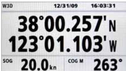
The nav data display shows receiver status, position in latitude and longitude (or TDs), course over ground, speed over ground, date and time.
