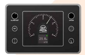
The THOR-120 is an echo sounder, connected via a P-120 sensor interface to a transducer. The echo sounder can be set to 0-4 and 0-40 meters. Between 0 and 4 meters, an alarm can be set to warn the operator when the preset minimum depth is reached. The THOR-120 echo sounder is specifically designed for use in shallow water, making it the ideal depth gauge for commercial inland shipping. The information is indicated on an analog indicator and a digital indicator.
